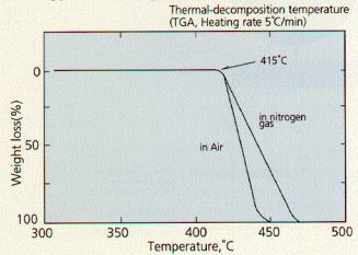
AFLAS provides excellent thermal stability. The copolymer starts to decompose in open-air or in nitrogen gas only at above 400°C.
